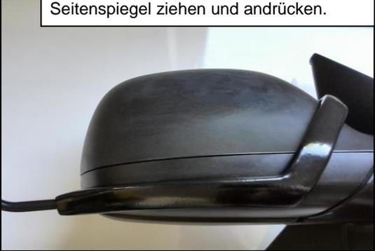
A close-up photograph showing the black mirror housing from a side profile. The black plastic bracket is being slid over the top edge of the housing. The bracket is positioned so that it will clamp onto the housing.
